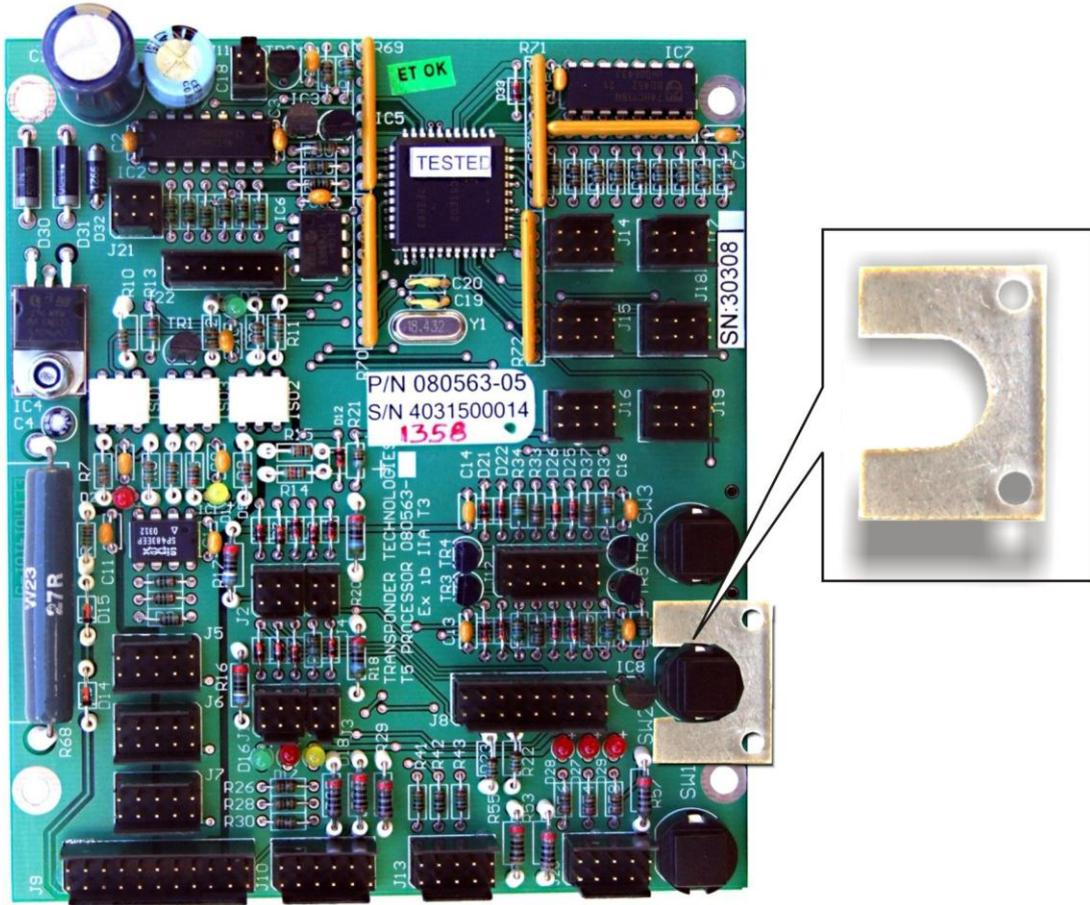
**Figure 3: Main Processor Board Switch Seal**
