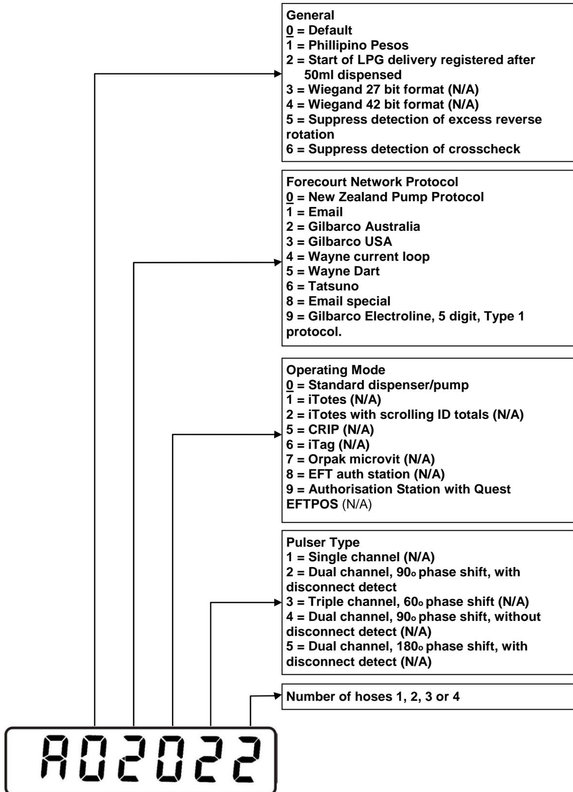
Each digit in this configuration parameter controls an aspect of the systems operation as shown below. This configuration factory set and should not be altered.
