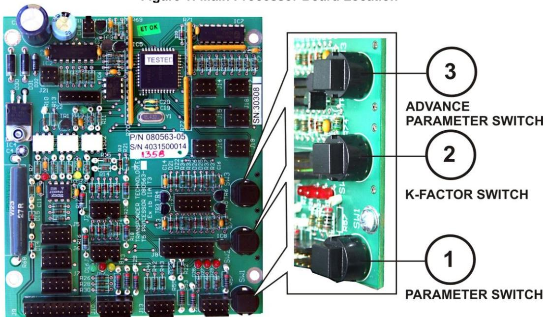
**Figure 2: Main Processor Board Switches**
